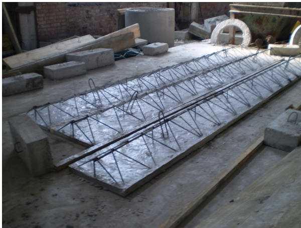
FIGURE 3. The look of framework slabs after manufacturing.
