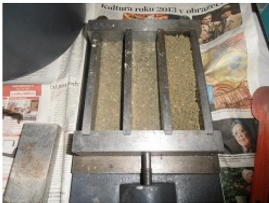
FIGURE 8. Production of the test specimens.
