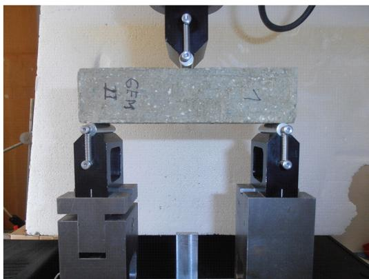
FIGURE 9. Three-point bend test.
