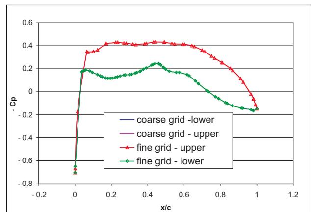
Fig. 7: Pressure distributions at the mid span for upper and lower surface
