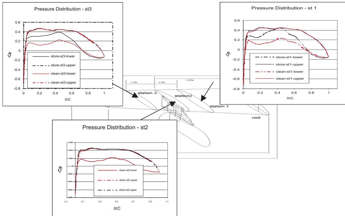
Fig. 8: Pressure distribution for a various chord wise location
