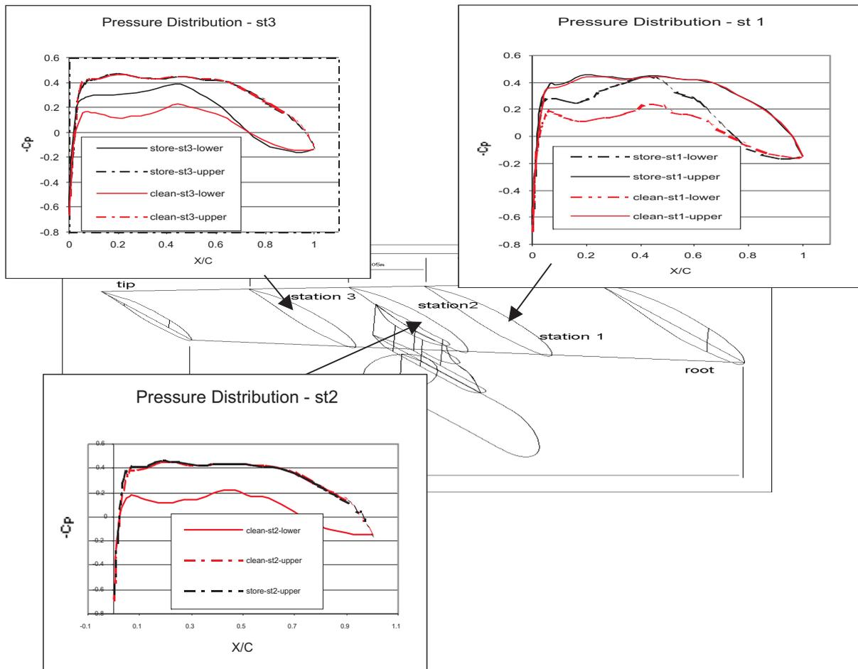
Fig. 9: Pressure coefficient at three different span wise locations
