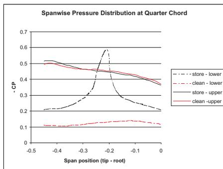
Fig. 10: External store interference on pressure distribution
