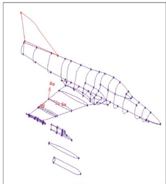
Fig. 3: Digitized wing geometry after smoothed with CAD
