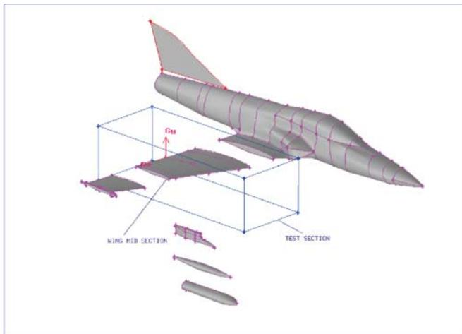
Fig. 4: Semi span model of a generic fighter aircraft
