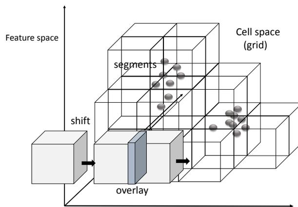
FIGURE 3. Cell space approximation in GRIDBSCAN classification. The dashed lines indicate the shift in the space with the overlap in which the clusters in the individual cells are interconnected.
