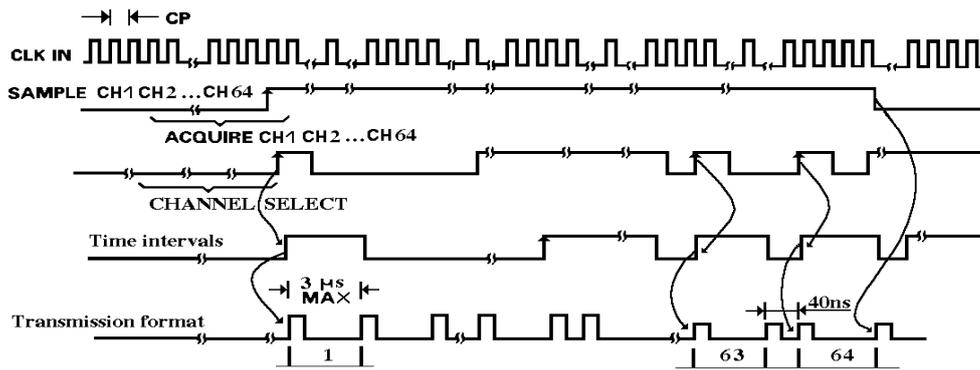
Fig. 2: Timing diagram of the sampling period
