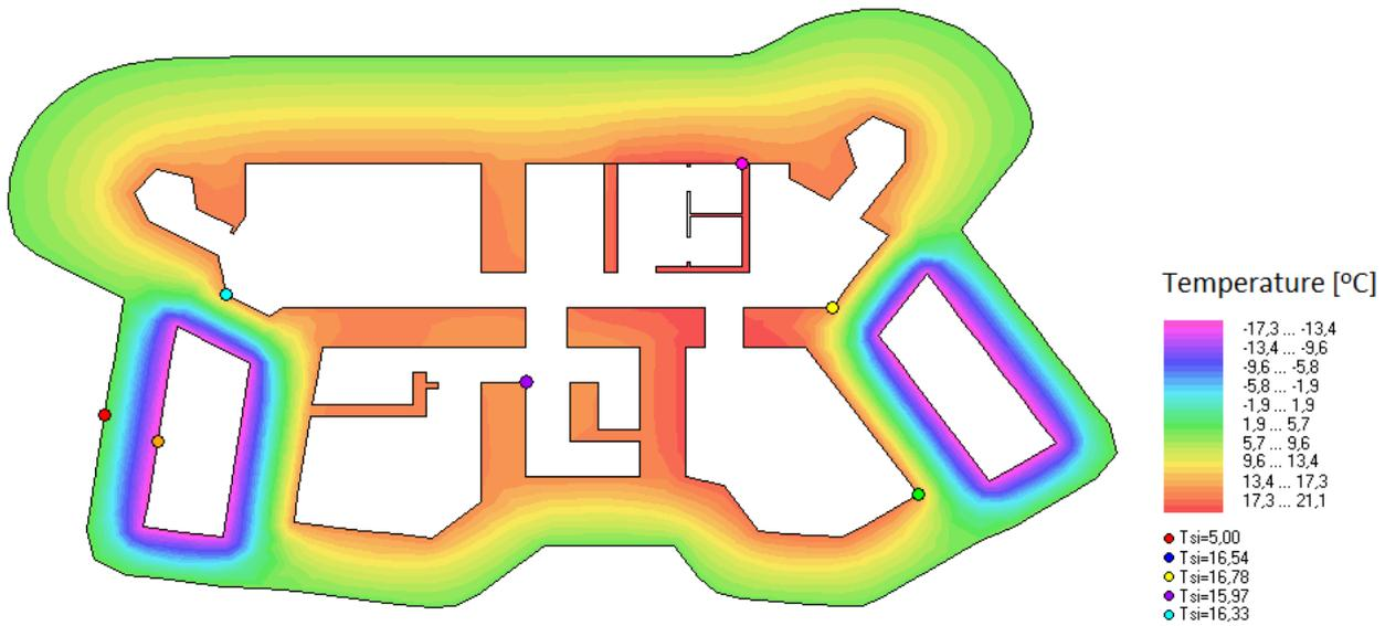
FIGURE 13. 2D thermal performance model of the underground floor (Area 2017).
