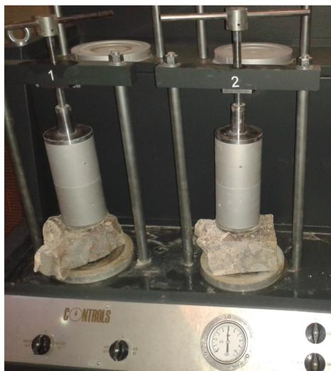
FIGURE 16. Sample from the bunker R-S-73 under the water penetration test (EN 12390-8).
