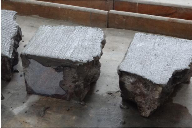
FIGURE 6. Samples with an applied crystallizing coating.
