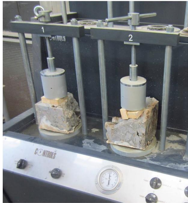
FIGURE 7. Samples with a crystallizing coating under the water penetration test (EN 12390-8).
