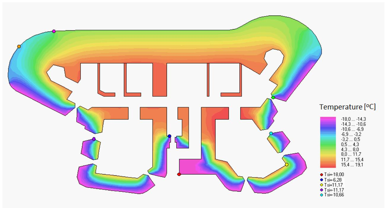
FIGURE 12. 2D thermal performance model of the first floor (Area 1717).
