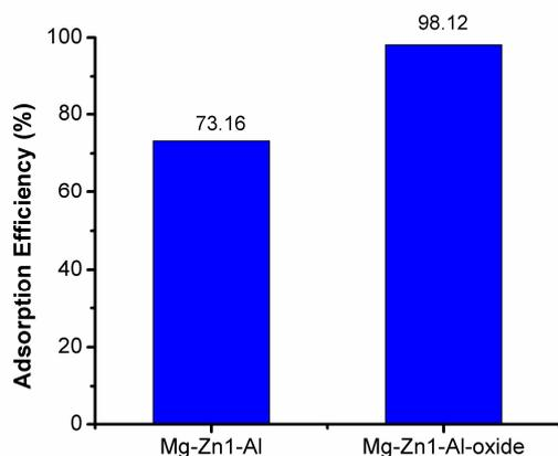
FIGURE 6. Adsorption efficiency of Mg-Zn1-Al HT and Mg-Zn1-Al HT oxide to  $Pb^{2+}$  metal ion.
