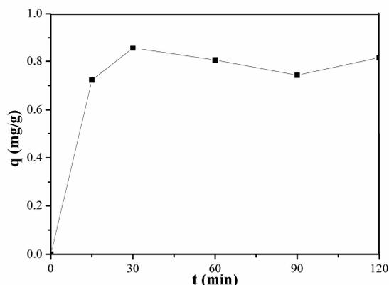
FIGURE 8. Effect of contact time on  $Pb^{2+}$  metal adsorption efficiency.
