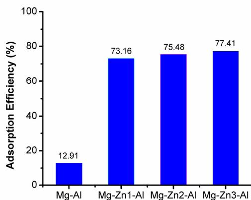
FIGURE 3. The effect of  $Zn^{2+}$  addition on the structure of Mg-Al HT on  $Pb^{2+}$  metal ions adsorption.
