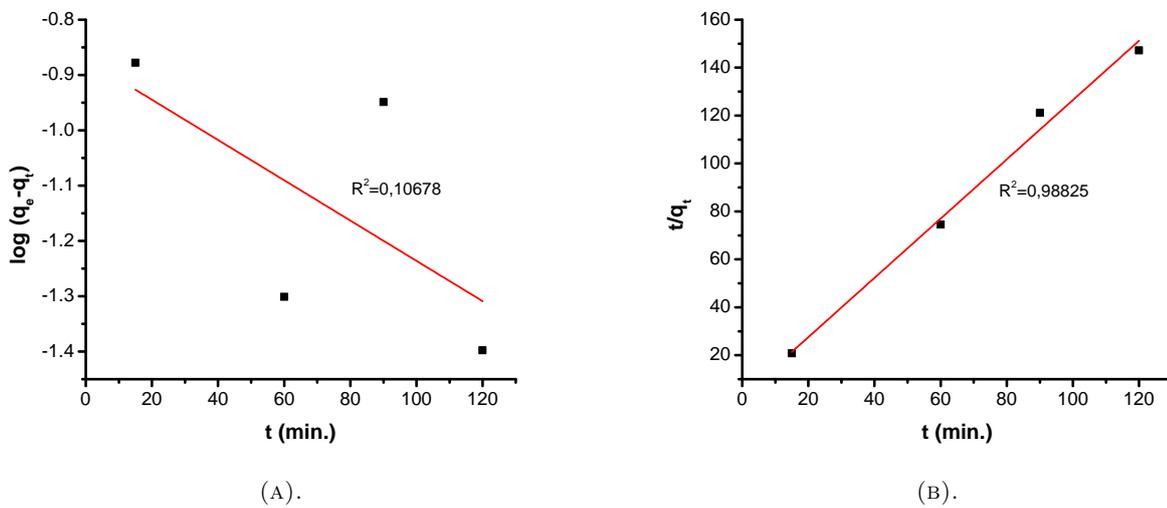
FIGURE 13. Adsorption kinetics curve of (a) pseudo first order and (b) pseudo second order.
