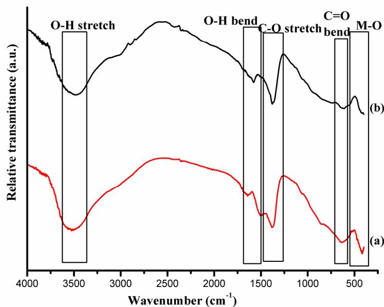
FIGURE 10. The functional group of Mg-Zn-Al HT oxide adsorbent (a) before and (b) after adsorption.
