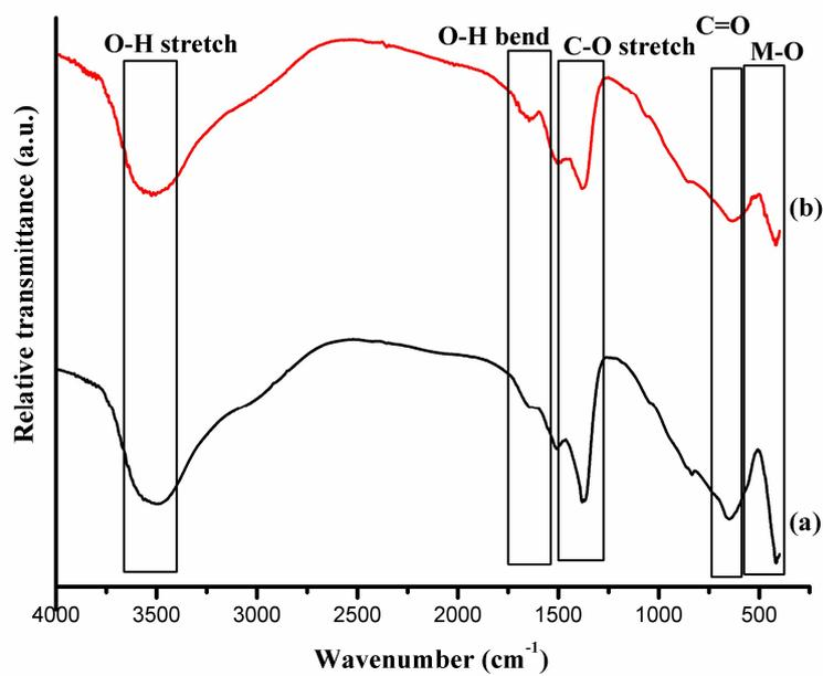
FIGURE 5. The FTIR spectrum of (a) Mg-Zn-Al HT and (b) Mg-Zn-Al HT oxide.
