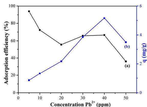
FIGURE 9. Effect of initial concentration on  $Pb^{2+}$  metal adsorption on (a) adsorption efficiency and (b) adsorption capacity.
