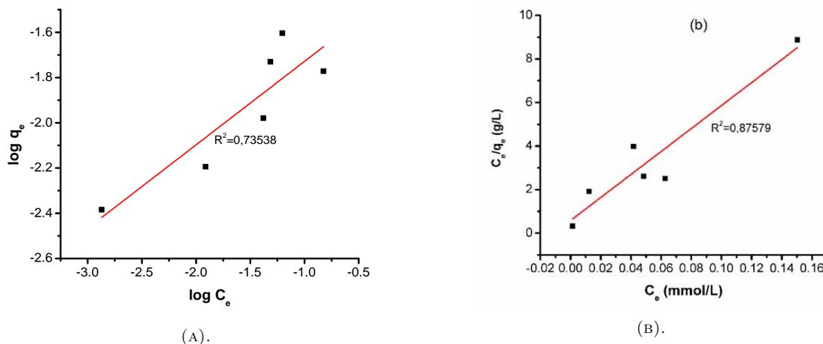
FIGURE 14. Adsorption isotherm curve of (a) Freundlich and (b) Langmuir.
