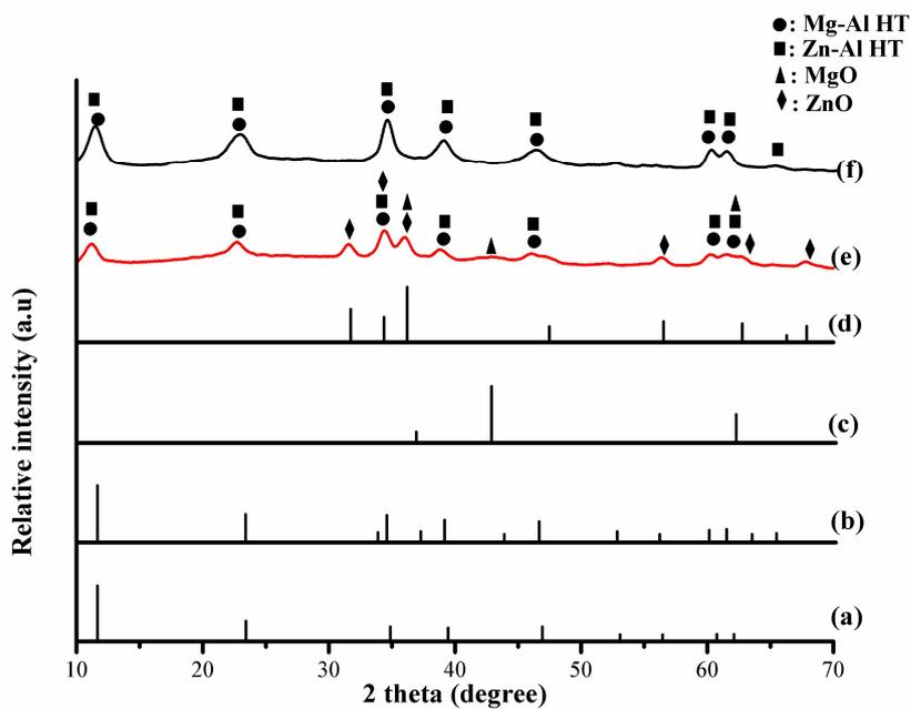
FIGURE 11. Diffractogram of (a) JCPDS Mg-Al HT (b) JCPDS Zn-Al HT (c) JCPDS MgO (d) JCPDS ZnO (e) Mg-Zn-Al HT oxide before adsorption and (f) Mg-Zn-Al HT oxide after adsorption.
