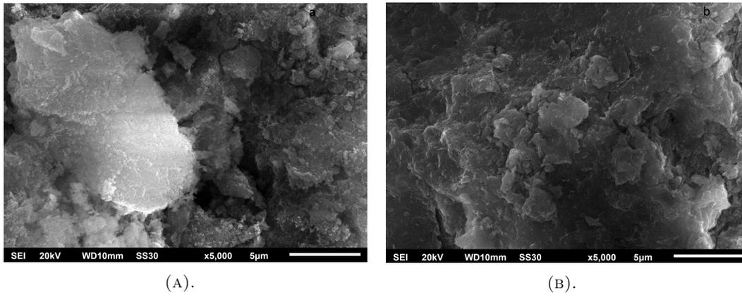
FIGURE 12. Morphology of Mg-Zn-Al HT (a) before and (b) after adsorption.
