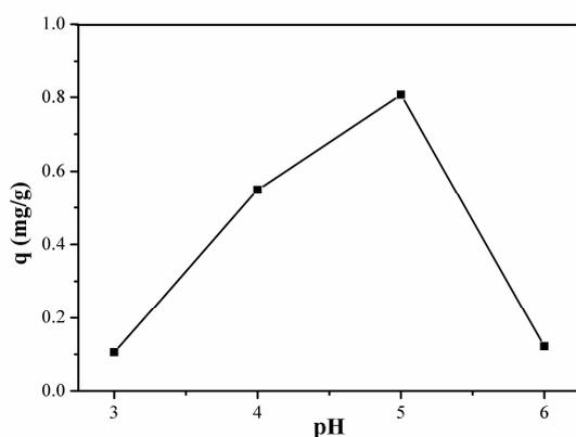
FIGURE 7. Effect of pH on  $Pb^{2+}$  metal adsorption efficiency.
