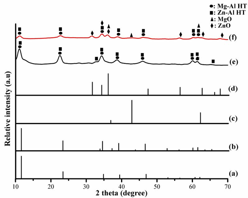
FIGURE 4. The diffractogram of (a) JCPDS Mg-Al HT (b) JCPDS Zn-Al HT (c) JCPDS MgO (d) JCPDS ZnO (e) Mg-Zn-Al HT and (f) Mg-Zn-Al HT oxide.
