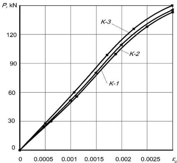
FIGURE 5. “ $P - \epsilon_c$ ” relations for K- 1(2, 3) set of columns.
