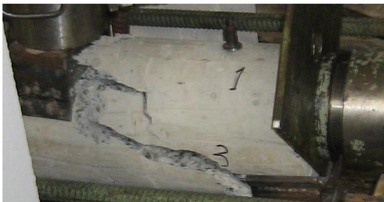
FIGURE 9. Pre-stressed column fracture along an oblique section.
