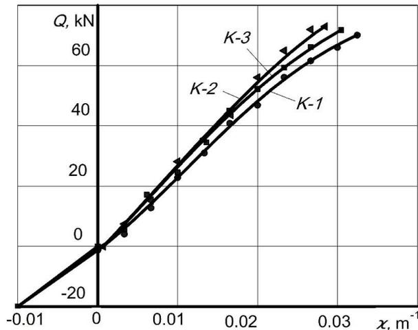
FIGURE 7. “ $Q - \chi$ ” relations of the CCSC under the conditions of longitudinal-transverse bending at  $a = 2\varnothing$  section bay, K- 1(2, 3) set.
