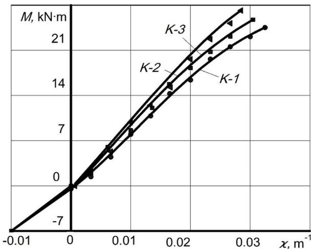
FIGURE 8. “ $M - \chi$ ” relations of the CCSC under the conditions of longitudinal-transverse bending at  $a = 2\varnothing$  section bay, K- 1(2, 3) set.
