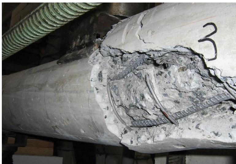
FIGURE 10. Dowel action in longitudinal tension reinforcement in terms of containing transverse shear of a CCSC.
