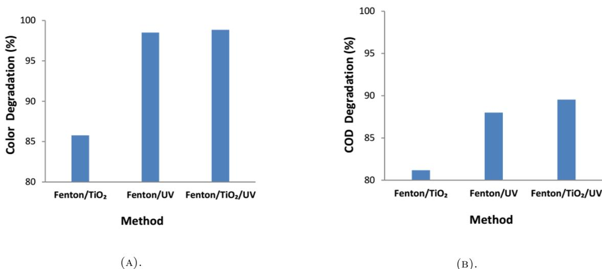
FIGURE 3. (a) RR 2 colour degradation and (b) COD removal by Fenton/TiO<sub>2</sub>, Fenton/UV, and Fenton/TiO<sub>2</sub>/UV methods (Fenton reagent molar ratio of 1 : 80, RR 2 concentration of 150 ppm, TiO<sub>2</sub> concentration of 0.4 %, pH 3, reaction time of 5 min).
