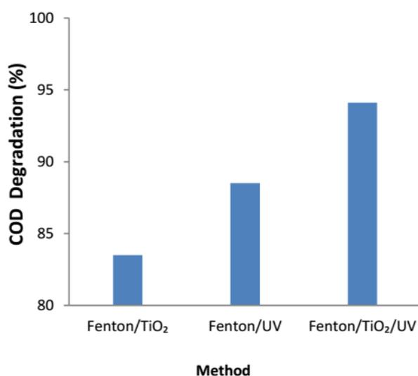
FIGURE 4. COD removal from the Jumputan fabric wastewater using Fenton/TiO<sub>2</sub>, Fenton/UV, and Fenton/TiO<sub>2</sub>/UV methods (Fenton reagent molar ratio of 1 : 80, pH of 3, 0.4 % TiO<sub>2</sub> catalyst concentration, reaction time of 120 min).
