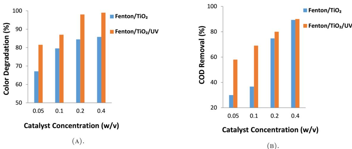
FIGURE 2. Effect of TiO<sub>2</sub> catalyst concentration on (a) RR 2 colour degradation and (b) COD removal by Fenton/TiO<sub>2</sub> and Fenton/TiO<sub>2</sub>/UV methods (Fenton reagent molar ratio of 1 : 80, RR 2 concentration of 150 ppm, pH 3, reaction time of 5 min).
