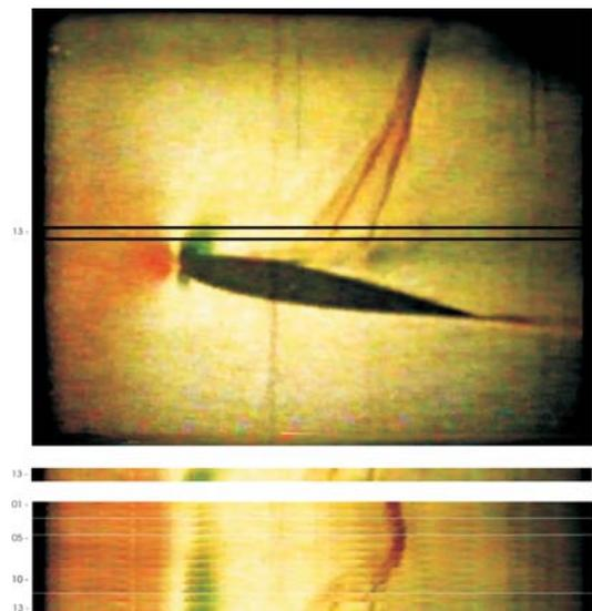
Fig. 3: Principle of the Colour Streak Schlieren Method
