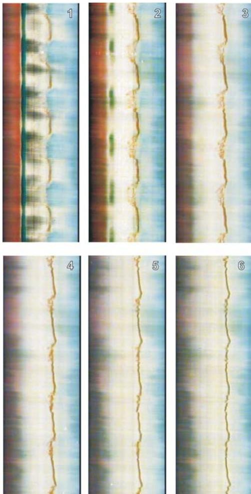
Fig. 8: CSSM pictures of terminal shock wave oscillation above the NACA 0012 airfoil
