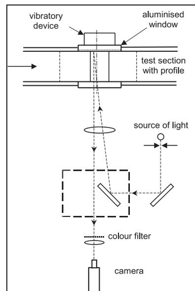
Fig. 1: Optical arrangement for schlieren method – oscillating profile configuration
