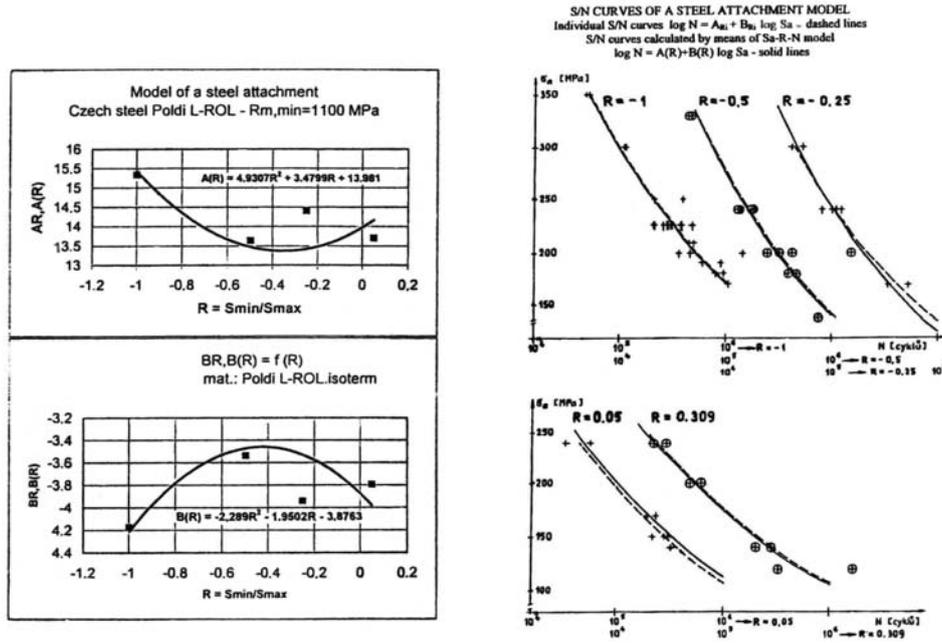
Fig. 3: The original test results for the test specimen that represents a steel attachment critical point
