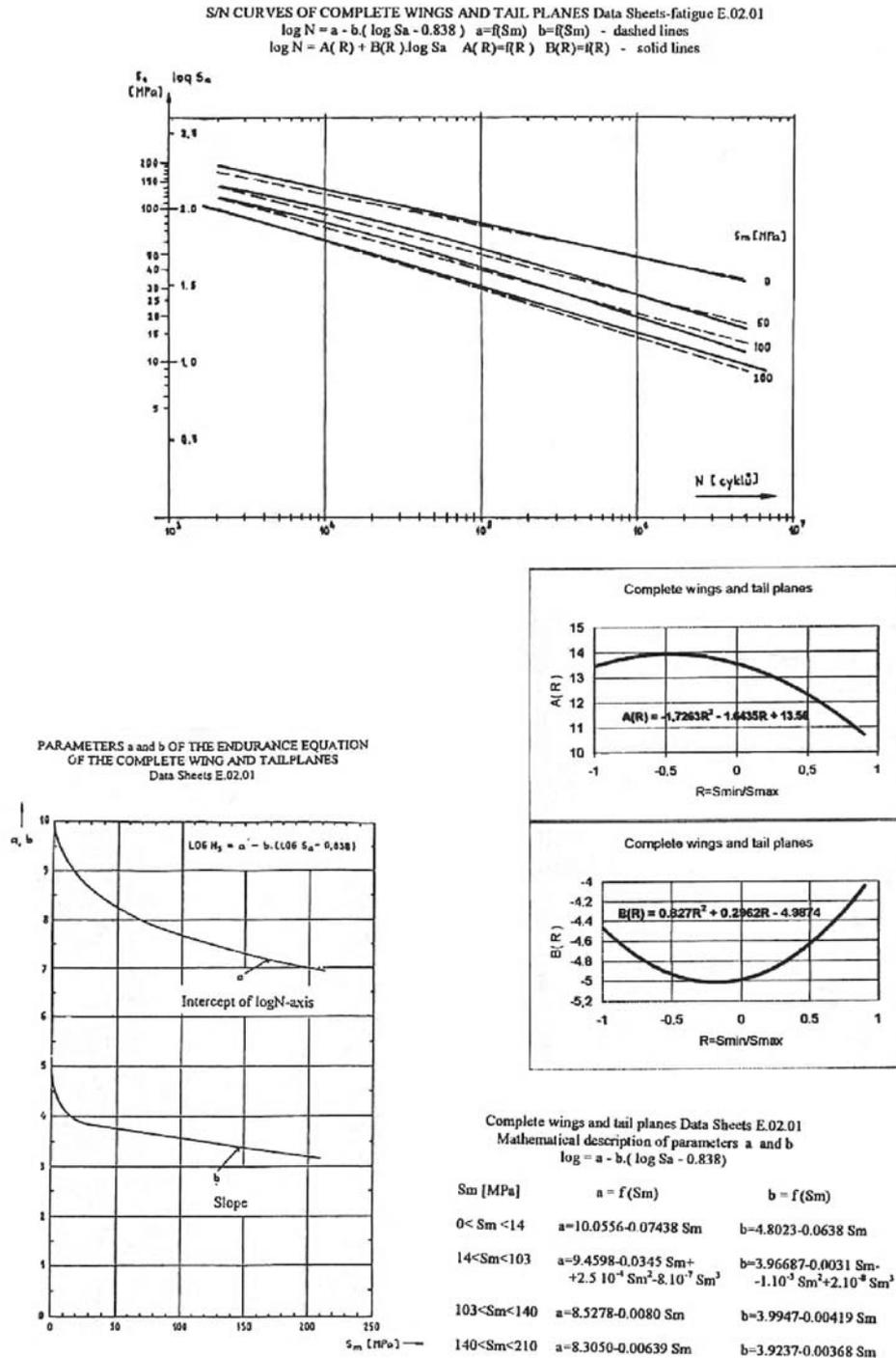
Fig. 1: S/N curves of complete wings and tail plans
