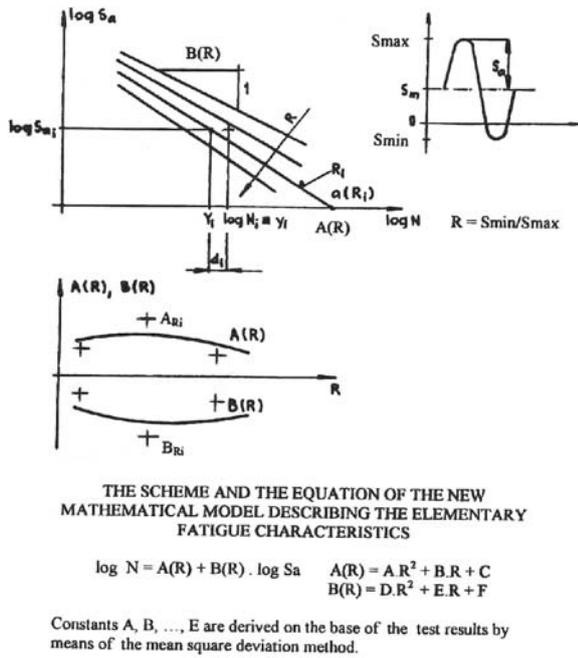
Fig. 2: The scheme and the equation of the new mathematical model describing the elementary fatigue characteristics
