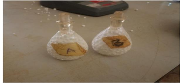
FIGURE 1. Polystyrene beads in pycnometer.
