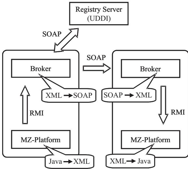
Fig. 4: Architecture of remote component
