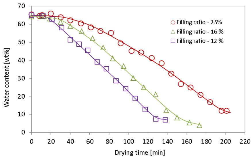
FIGURE 3. Drying curves for various filling ratio.
