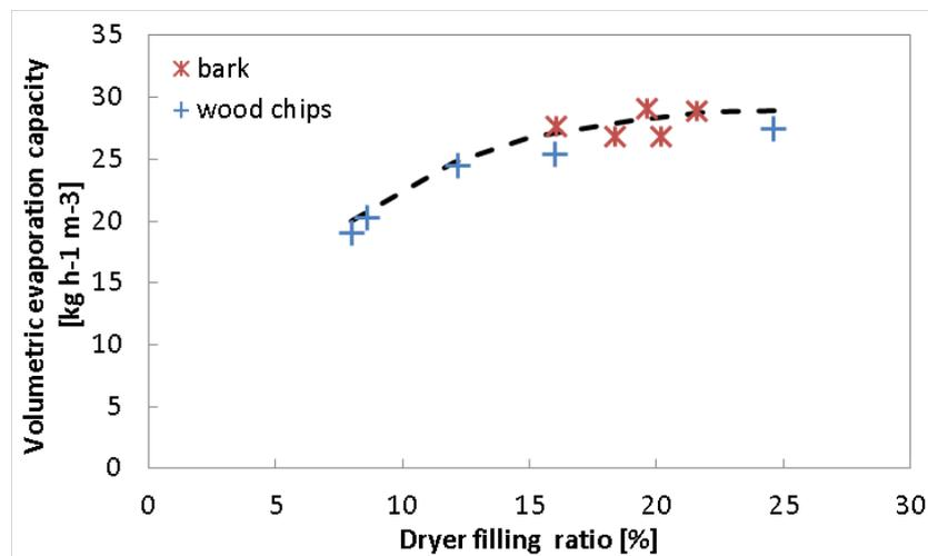
FIGURE 5. Volumetric evaporation capacity in the dependence on the drum filling ratio.
