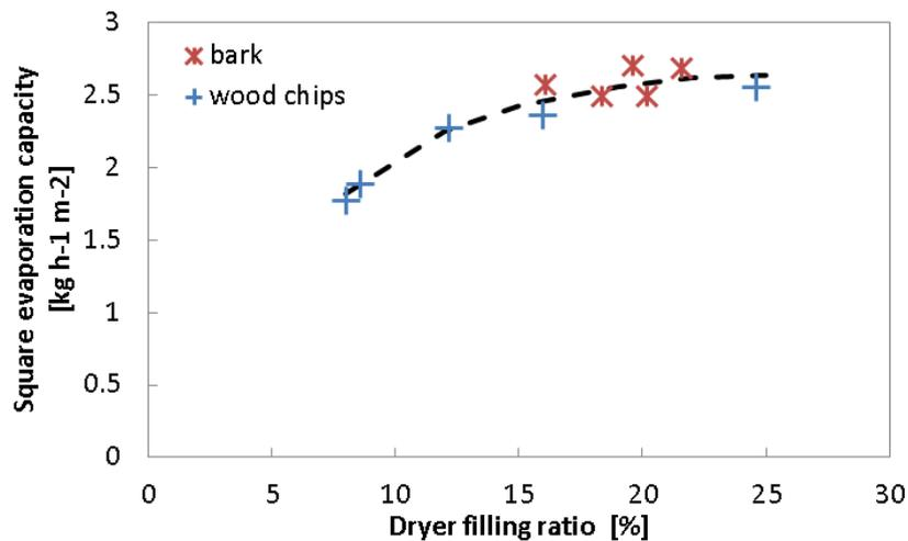
FIGURE 4. Square evaporation capacity in the dependence on the drum filling ratio.
