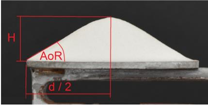
FIGURE 1. Scheme of measurement of  $AoR$  (Fine glass bead particles).
