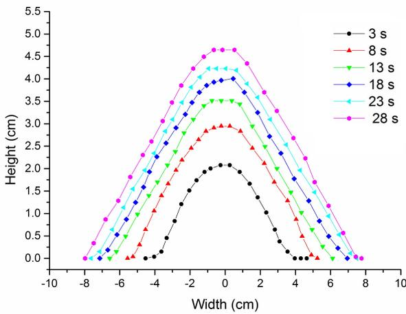
FIGURE 12. Evolution of  $AoR$  during tests with 8 mm funnel.
