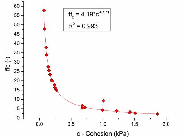
FIGURE 10. Influence of cohesion on flow function parameter.
