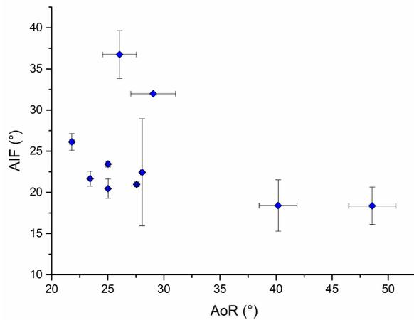
FIGURE 9. Comparison between Angle of Internal friction ( $AIF$ ) and  $AoR$ .
