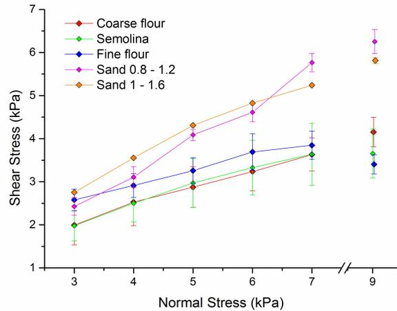
FIGURE 6. Shear Cell Test of sands, flours and semolina.
