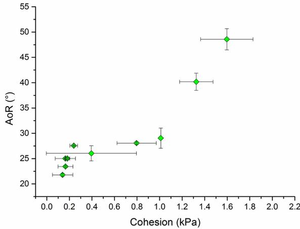
FIGURE 8. Influence of cohesion ( $c$ ) on  $AoR$ .
