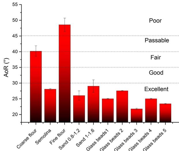
FIGURE 2. Values of  $AoR$  for different experimental material.
