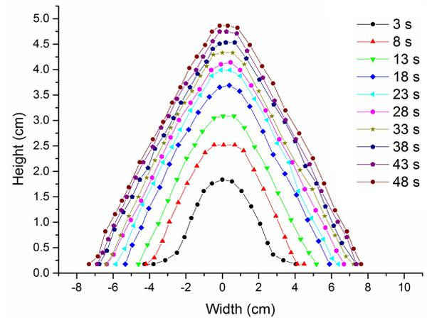
FIGURE 11. Evolution of  $AoR$  during tests with 5 mm funnel.
