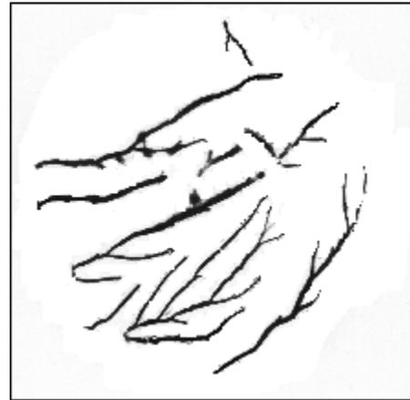
Fig. 2: Surface streamers extracted from Fig. 1
