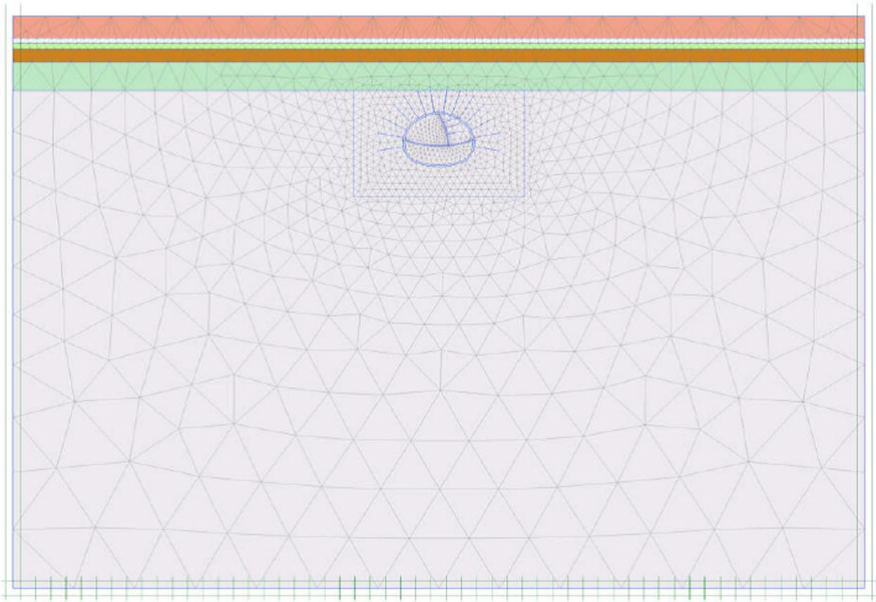
FIGURE 4. Finite element mesh with horizontal tunnel face sequencing.
