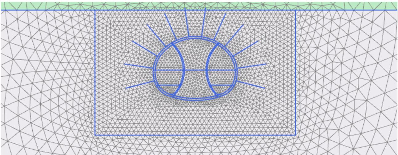
FIGURE 5. Detail of finite element mesh with vertical tunnel face sequencing.
