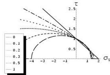
Fig. 7: Coulomb for the maximum shear plane  $\tan \varphi = 0.5$ , ( $\varphi = 26.6^\circ$ ),  $c = 1$  and several values of parameter  $\mu$
