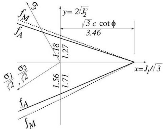
Fig. 3: The modified Coulomb (A) and the original Mohr-Coulomb (M) for  $\tan \varphi = 0.5, (\varphi = 26.6^\circ), c = 1$  in the rendulic plane  $\sigma_1 = \sigma_2$ . Axis  $\sigma_1$  and projection of axes  $\sigma_1$  and  $\sigma_2$  are also shown.
