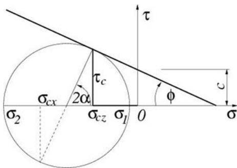
Fig. 1: Inclination  $\alpha$  of the critical plane in the classical Mohr-Coulomb yield condition
