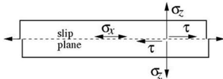
Fig. 4: Stress components at yield in the direct shear test
