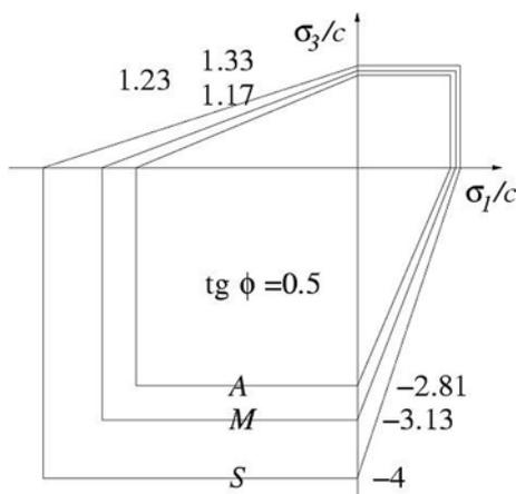
Fig. 2: The modified Mohr-Coulomb (A), the original Mohr-Coulomb (M) and the maximum shear plane condition (S) for  $\tan \varphi = 0.5, \varphi = 26.6^\circ$
