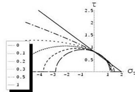
Fig. 6: Modified Mohr-Coulomb for  $\tan \varphi = 0.5$ , ( $\varphi = 26.6^\circ$ ),  $c = 1$  and several values of parameter  $\mu$
