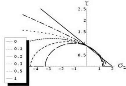
Fig. 5: Mohr-Coulomb for  $\tan \varphi = 0.5$ , ( $\varphi = 26.6^\circ$ ),  $c = 1$  and several values of parameter  $\mu$
