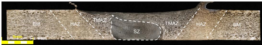
FIGURE 2. Macrostructure of T81 joint.
