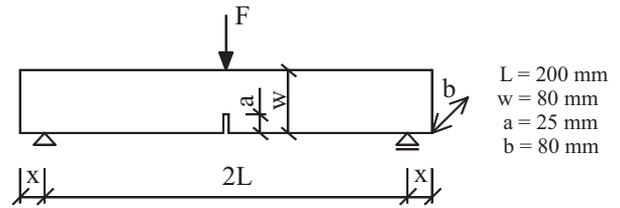
Fig. 4: Notched beam under three-point bending
