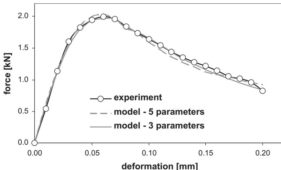
Fig. 6: Load deflection curves – experiment and numerical simulation using identified parameters
