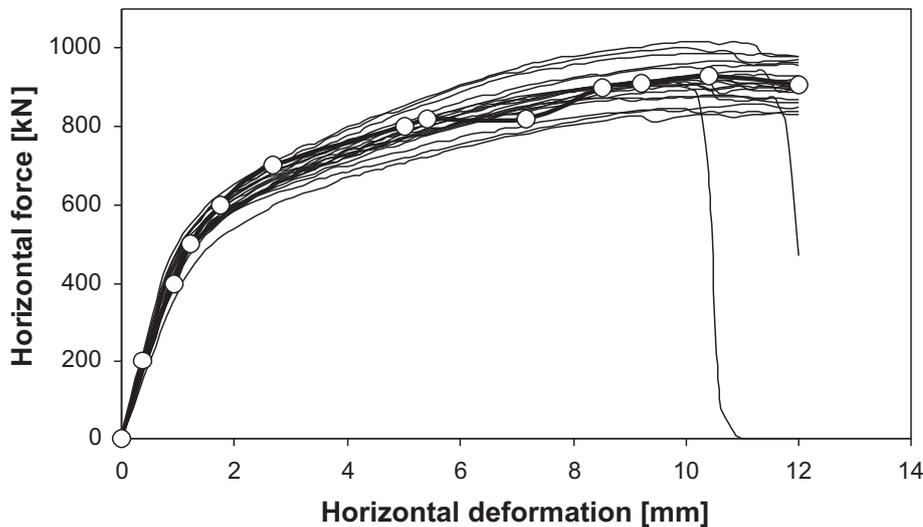
Fig. 8: Random load-deflection curve realizations – 20 simulations of LHS
