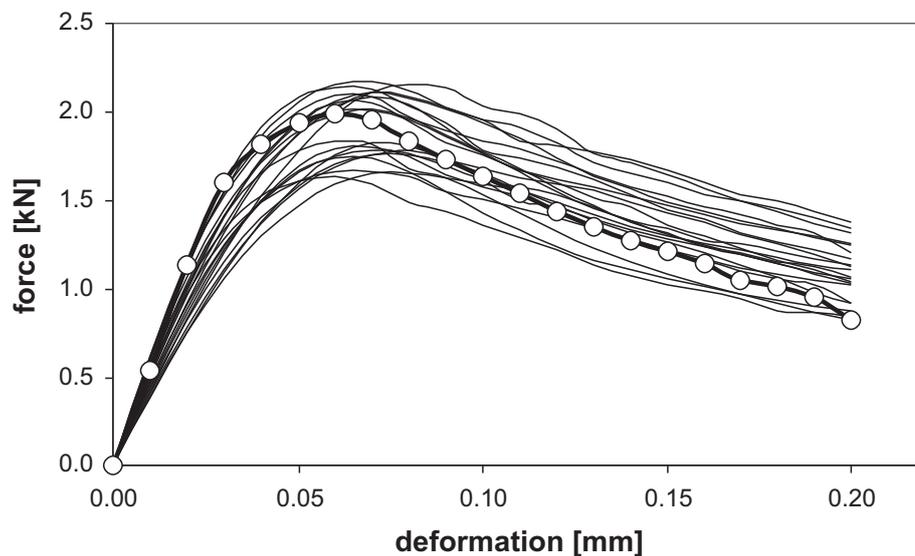
Fig. 5: Random load-deflection curve realizations – 20 simulations of LHS
