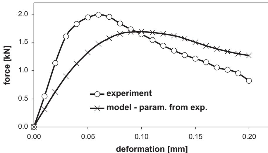
Fig. 1: Load-deflection curves – experiment and initial numerical simulation
