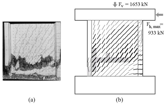
Fig. 7: Shear wall experimental failure and its ATENA simulation: (a) experimental failure, (b) failure simulated by ATENA
