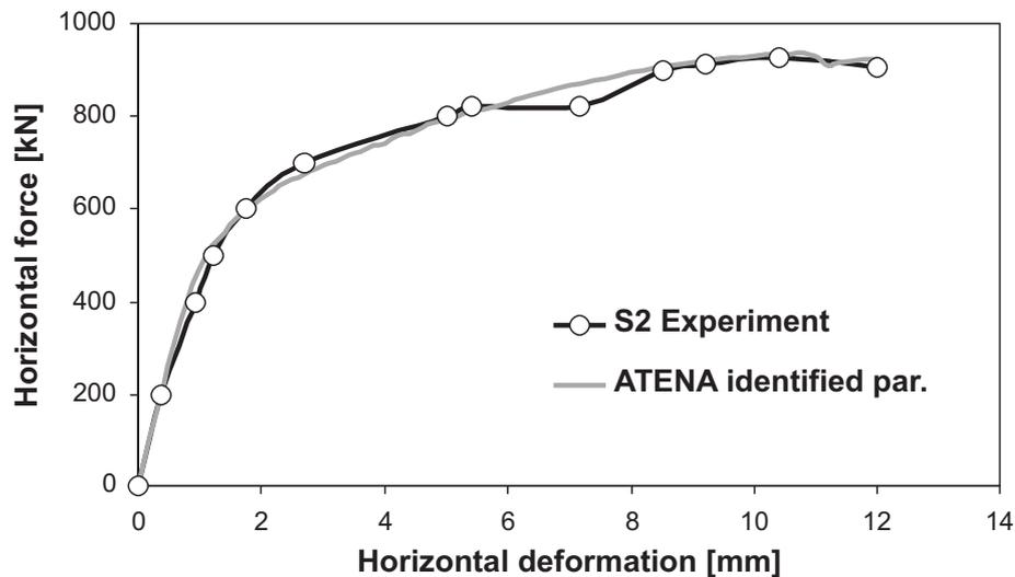
Fig. 9: Load deflection curves – experiment and simulation using identified parameters
