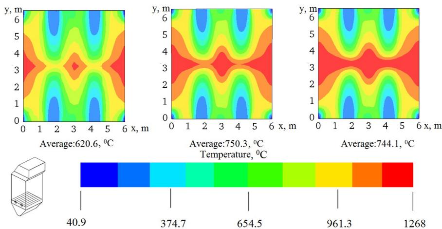
FIGURE 4. Temperature distribution in the area of burner arrangement for various percentages of air supplied through injectors: a) OFA = 0% (basic version), b) OFA = 10%, c) OFA = 18%.
