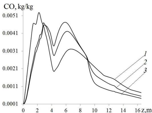
FIGURE 9. The distribution of the concentration of carbon monoxide CO at the outlet of the combustion chamber of the boiler BKZ-75 at various percentages of air supplied through OFA injectors: a) OFA = 0% (basic version), b) OFA = 10%, c) OFA = 18%.
