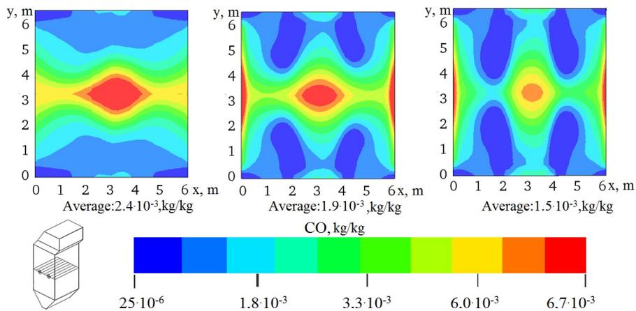
FIGURE 8. The distribution of the concentration of carbon monoxide CO in the area of the location of OFA injectors at various percentages of air supplied through injectors: a) OFA = 0% (basic version), b) OFA = 10%, c) OFA = 18%.
