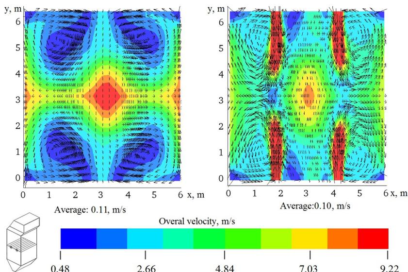
FIGURE 3. The field of the overall velocity vector in the region of the arrangement of OFA injectors for various percentages of air supplied through injectors: a) OFA = 0% (basic version), b) OFA = 10%.
