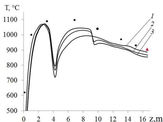
FIGURE 6. Temperature distribution  $T$  along the height of the combustion chamber of the boiler BKZ-75 at various percentages of air supplied through injectors OFA: 1 – OFA = 0% (basic version), 2 – OFA = 10%, OFA = 18%; “black circle” – experiment at TPP [49]; “red triangle” – is theoretical values obtained by the method of thermal calculation CBTI – Central Boiler-and-Turbine Institute [50].
