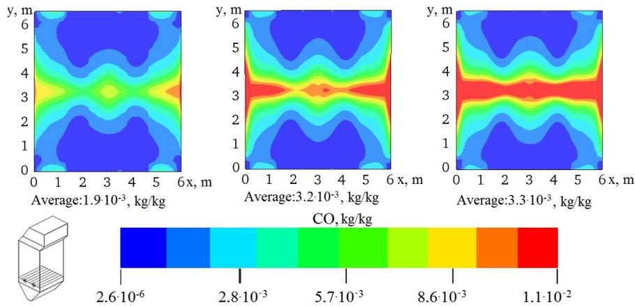
FIGURE 7. The distribution of the concentration of carbon monoxide CO in the area of the location of the burners for different volumes of air supplied through the injectors: a) OFA = 0% (basic version), b) OFA = 10%, c) OFA = 18%.
