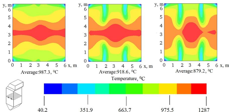
FIGURE 5. Temperature distribution in the area of the location of OFA injectors for various percentages of air supplied through injectors: a) OFA = 0% (basic version), b) OFA = 10%, c) OFA = 18%.
