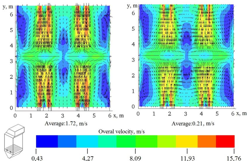
FIGURE 2. The field of the overall velocity vector in the area of the arrangement of the burners for various percentages of air supplied through the injectors: a) OFA = 0% (basic version), b) OFA = 10%.
