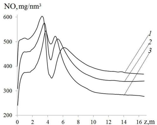
FIGURE 10. Distribution of the concentration of nitrogen oxide NO along the height of the combustion chamber of the BKZ-75 boiler at various percentages of air supplied through OFA injectors: a) OFA = 0% (basic version), b) OFA = 10%, c) OFA = 18%.
