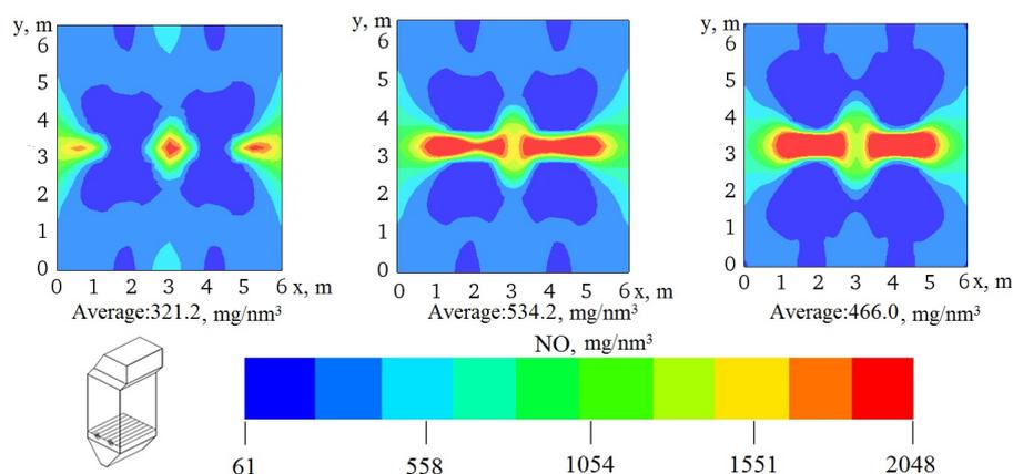
FIGURE 11. The distribution of the concentration of nitrogen oxide NO in the area of the burners for different volumes of air supplied through OFA injectors: a) OFA = 0 % (basic version), b) OFA = 10 %, c) OFA = 18 %.
