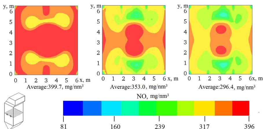
FIGURE 12. The distribution of the concentration of nitrogen oxide NO in the area of OFA injectors at various percentages of air supplied through injectors: a) OFA = 0 % (basic version), b) OFA = 10 %, c) OFA = 18 %.
