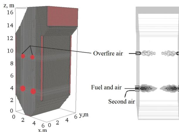
FIGURE 1. General view of the combustion chamber of the BKZ-75 boiler of the Shakhtinskaya TPP, a) its breakdown into control volumes and b) the layout of OFA burners and injectors.
