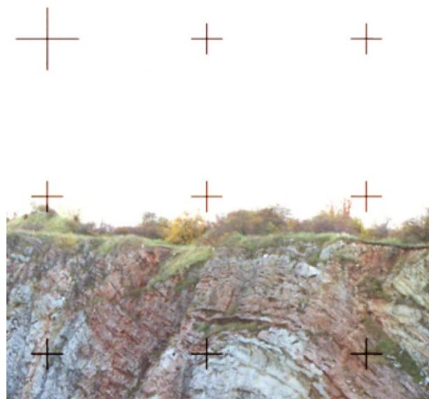
FIGURE 2. Part of an image with projected reference points of réseau plate.
