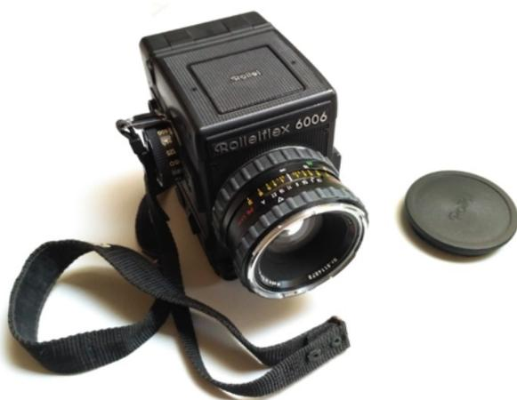
FIGURE 1. Camera Rollei 6006 metric.
