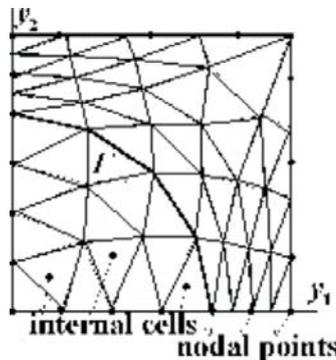
Fig. 2: Geometry of boundary elements and internal cells
