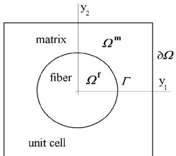
Fig. 1: The unit cell – geometry and denotation
