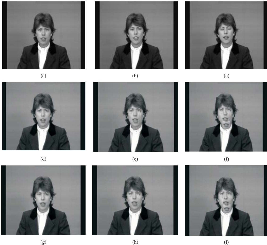
Fig. 6: (a) the original 2 nd frame, (b) the original 5 th frame, (c) the original 8 th frame, (d) reconstructed frame 2 using the FS algorithm, (e) reconstructed frame 5 using the FS algorithm, (f) reconstructed frame 8 using the FS algorithm, (g) reconstructed frame 2 using the TSS algorithm, (h) reconstructed frame 5 using the TSS algorithm, (i) reconstructed frame 8 using the TSS algorithm
