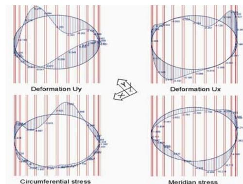
Fig. 2: Calculated deformations and stresses of the shell in the middle of the length; the values are obtained for diameter 400 mm, thickness 0.5 mm and length 2.0 m, and for loading by the wind downstream of axis Y
