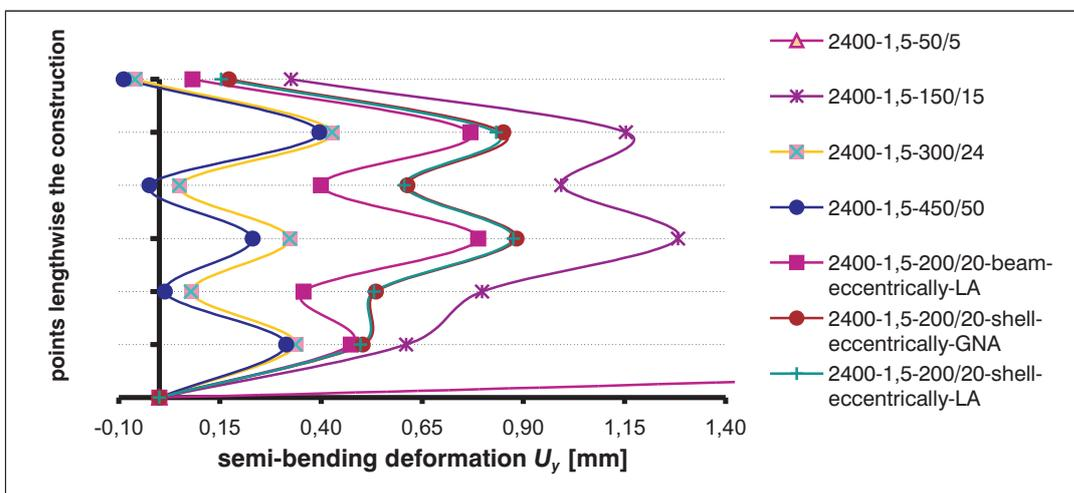
Fig. 9: Comparison of the lengthwise semi-bending deformation of the shell for one numerical model and a given stiffness of the stiffener on the side exposed to the wind
