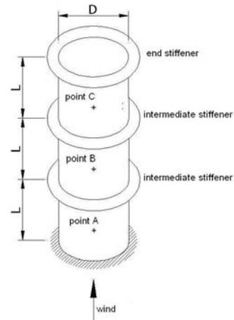
Fig. 6: Numerical model of the shell that was used for determining the optimum distance of the stiffeners. The stiffeners and the other investigated points are identified in the figure
