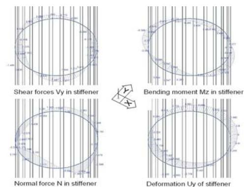
Fig. 7: Parameters of ring stiffener No. 2 for diameter of a cylindrical shell 1600 mm, thickness 3.0 mm and distance between stiffeners 4.0 m. Stiffeners of profile 300/24 (second moment  $5.4 \times 10^7 \text{ mm}^4$ ) and loading by wind downstream of axis  $Y$  are investigated.
