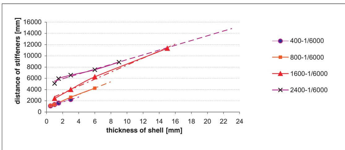
Fig. 3: Dependence of the maximum distance of the stiffeners on the thickness of the shell for diameter 400 mm, 800 mm, 1600 mm and 2400 mm, for limit deformation of the shell  $D/6000$
