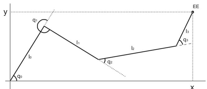
Fig. 1: Articulated structure with notation and numbering
