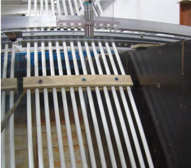
FIGURE 10. Movable attachments guaranteeing free length and rotation of the screen bars rods.
