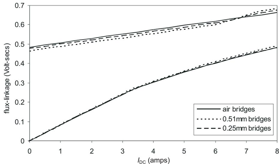
Fig. 12: Direct and quadrature axis magnetisation curves for one phase of test motor 2
