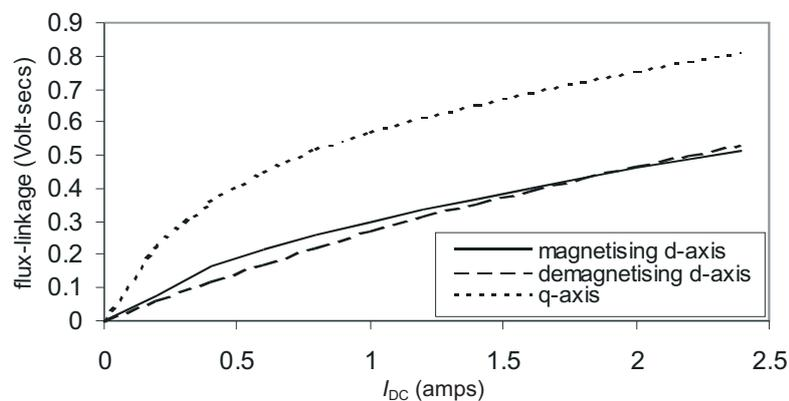
Fig. 5: Results of flux-linkage simulations for test motor 1 with remodelled rotor bridges
