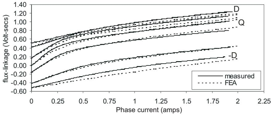
Fig. 3: Comparison between measured and FE-simulated magnetisation curves
