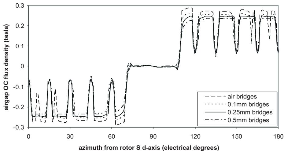
Fig. 10: Open circuit airgap flux density distribution of test motor
