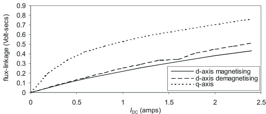
Fig. 4: Test motor 1 flux-linkages due to current
