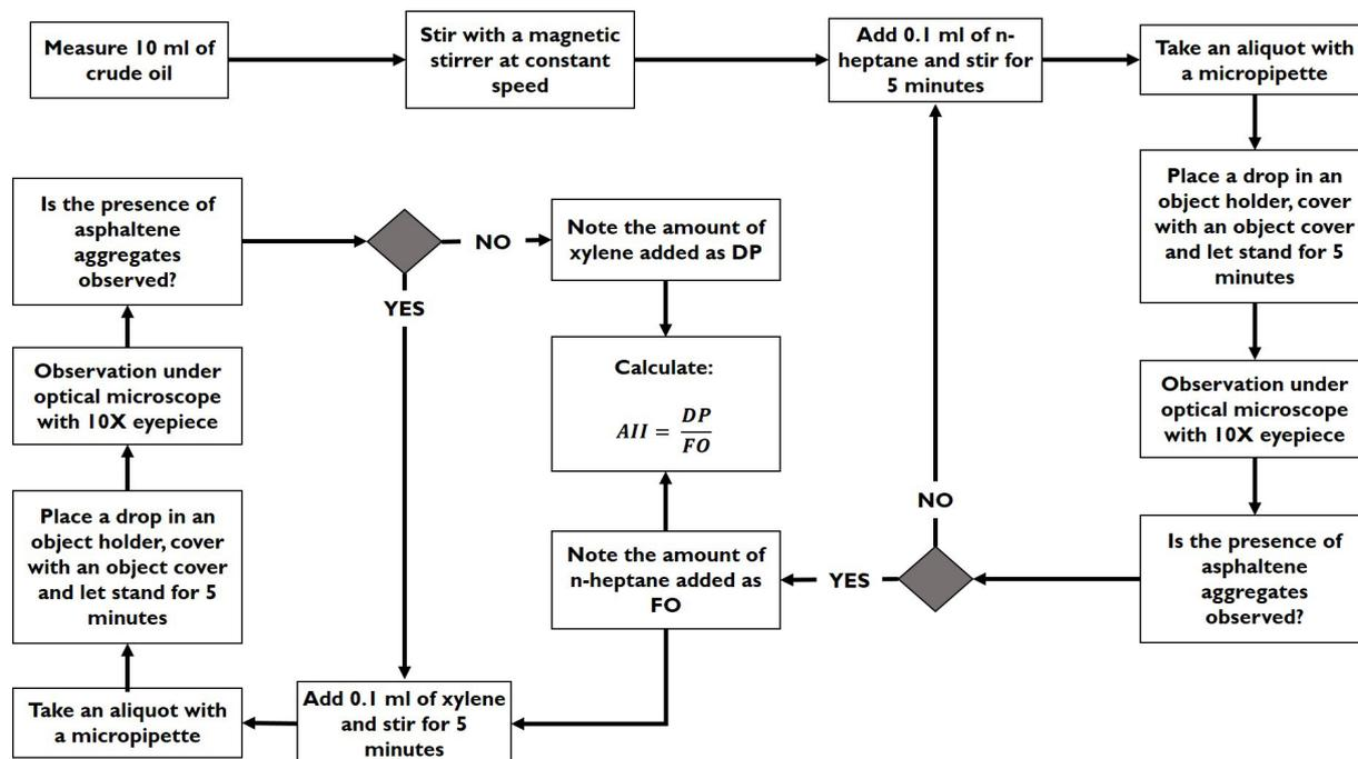
FIGURE 1. Flowchart of the procedure to obtain the AII.
