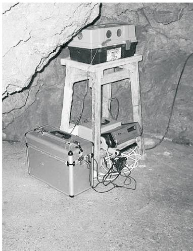
Fig. 3: Radim 3 continual radon monitor in a plastic box with dessiccant, AlphaGuard continual radon monitor, Fritra 4 continual radon and attached and unattached radon daughters fraction monitor
