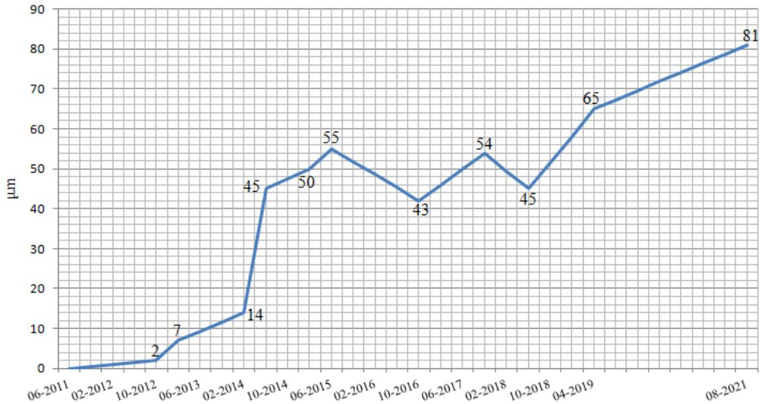
FIGURE 5. The difference of the additive constant of the Leica AT401 laser tracker and the Leica RRR 1.5 spherical prism in the period between June 2011 and August 2021.
