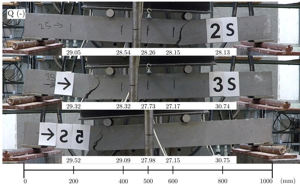
FIGURE 12. Cracking patterns compared with the non-destructive measurement results.
