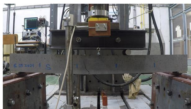
FIGURE 5. Four-point bending test setup.
