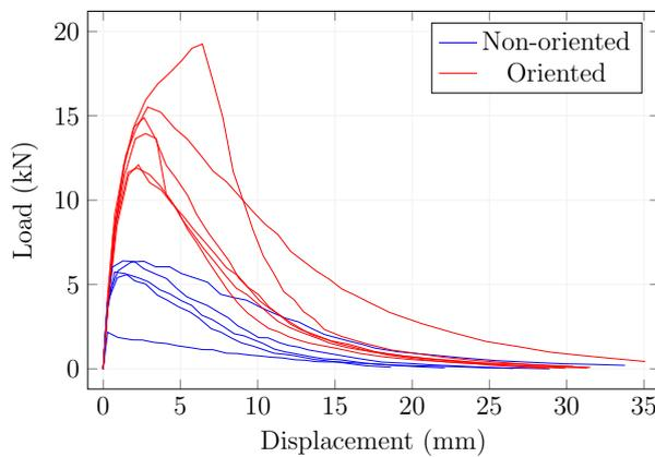
FIGURE 10. Load-displacement diagrams.
