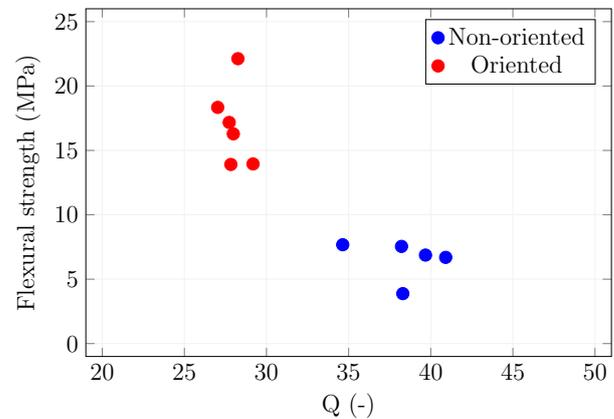
FIGURE 11. The quality factors  $Q$  compared to the measured flexural strengths for all specimens
