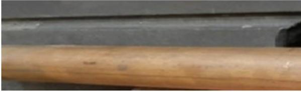
FIGURE 11. Outer surface of the inner pipe with plain profile.
