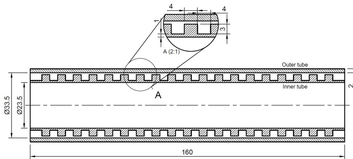
FIGURE 4. Dimensions of rectangular labyrinth heat exchanger.
