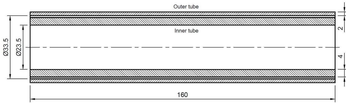
FIGURE 3. Dimensions of the plain heat exchanger.
