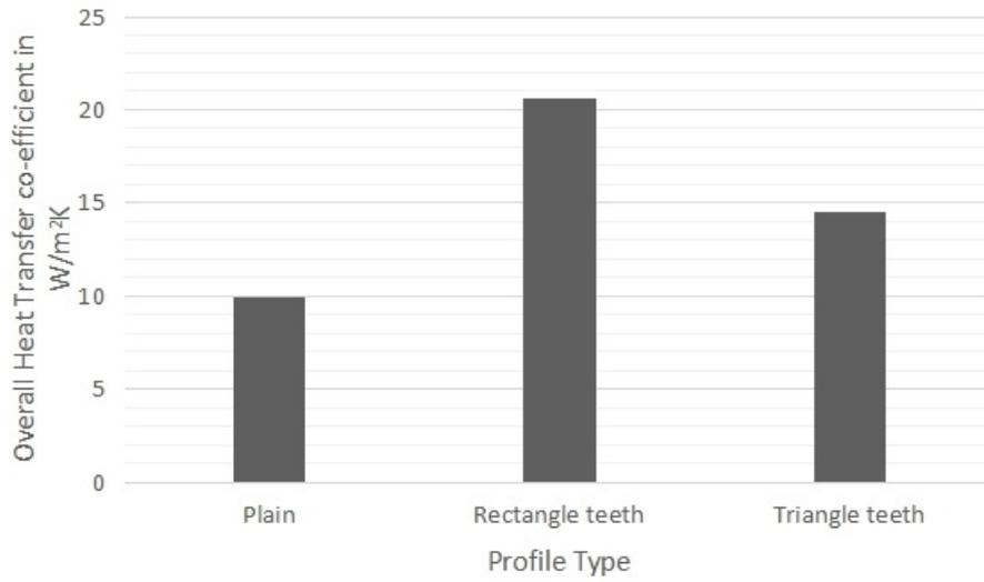
FIGURE 16. Comparison of overall heat transfer coefficient for CFD results.
