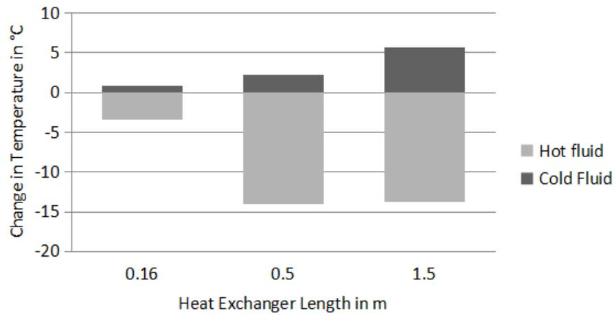
FIGURE 14. Effect of increasing the heat exchanger length (Hot fluid in inner pipe at 0.4 kg s<sup>-1</sup>).
