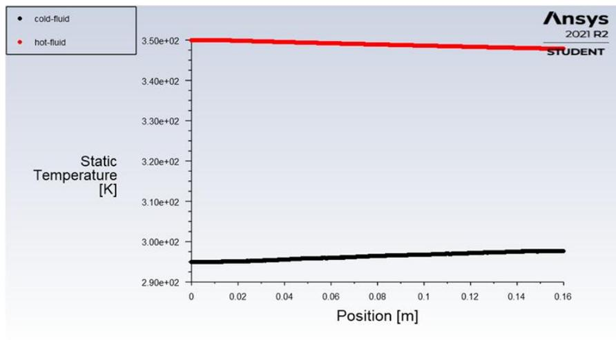
FIGURE 17. Temperature plot for plain heat exchanger.
