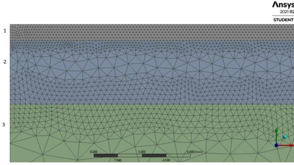
FIGURE 6. Mesh picture for plain heat exchanger model.
