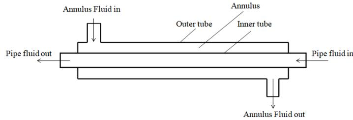
FIGURE 1. Schematic of the double pipe heat exchanger.
