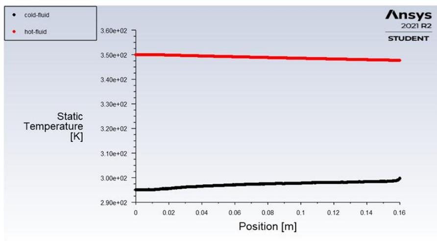
FIGURE 18. Temperature plot for rectangular labyrinth heat exchanger.
