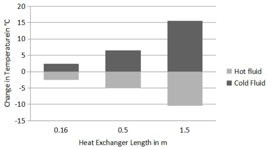
FIGURE 15. Effect of increasing the heat exchanger length (Hot fluid in inner pipe at 0.8 kg s<sup>-1</sup>).
