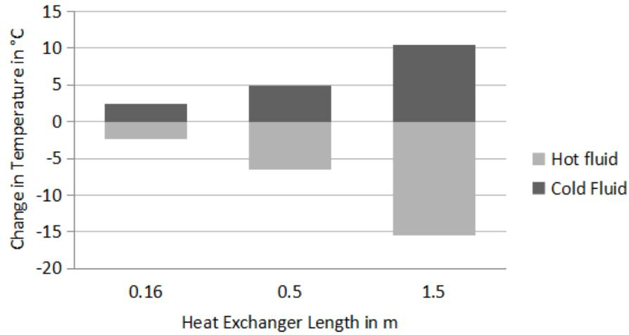
FIGURE 13. Effect of increasing the heat exchanger length (Hot fluid in annulus at 0.4 kg s<sup>-1</sup>).
