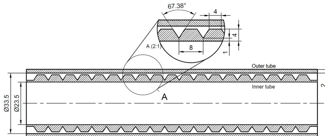
FIGURE 5. Dimensions of the triangular labyrinth heat exchanger.
