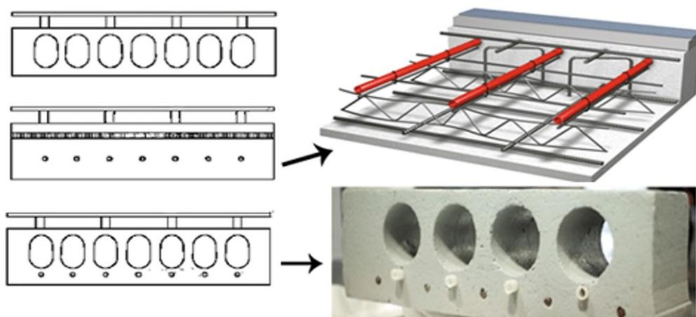
FIGURE 2. Division of TABS according to the position of the heat transfer medium: In the upper part: the heat transfer medium is air distributed through the cavities in the ceiling panel, in the middle: the heat transfer medium is a liquid in a pipe – monolithic ceiling, in the lower part: the heat transfer medium is a liquid in a pipe – prefabricated ceiling panel [5].
