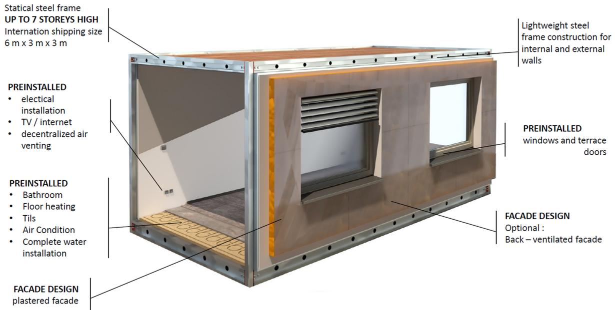
FIGURE 1. Standardised SUNOMAXCUBE building module with integrated energy-active elements in the building structures [4].
