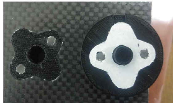
FIGURE 8. Insert after the installation with the use of adhesive tape.
