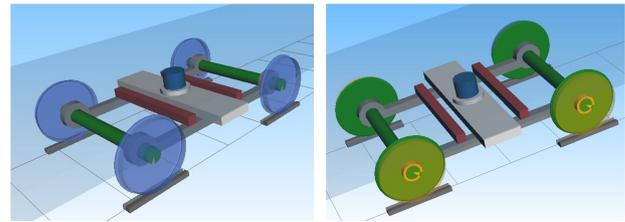
FIGURE 2. A railway running gear with the TKS wheels (left) and with the PKS wheels (right).
