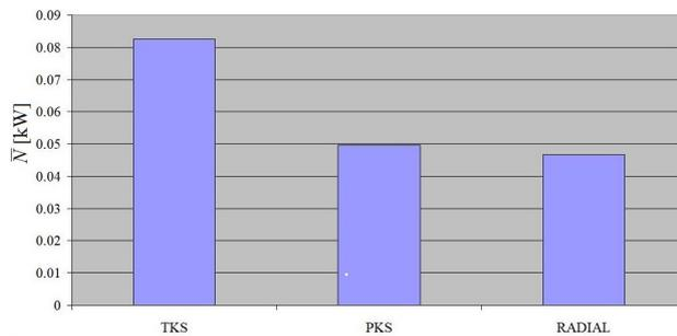
FIGURE 6. The average power  $\bar{N}$  [kW] dissipated when the wheels of the tram car slip on the rails during the passage of the considered route at a speed of  $10 \text{ km}\cdot\text{h}^{-1}$ ; TKS – a bogie with the traditional construction scheme, PKS – a bogie with the perspective construction scheme, RADIAL – a bogie with the radial setting system.
