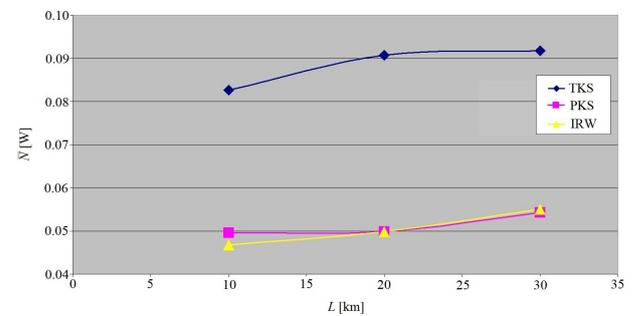
FIGURE 8. The value of the average power  $\bar{N}$  [kW] dissipated when the wheels of the tram cars slide on the rails during the passage of the considered route  $L$  [km]; TKS – a bogie with the traditional construction scheme, PKS – a bogie with the perspective construction scheme, RADIAL – a bogie with the radial setting system.
