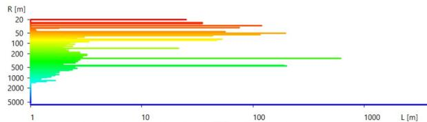
FIGURE 1. A bar graph of the curved sections of the route.
