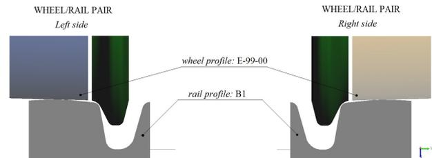
FIGURE 3. A visualisation of the contact zone of a wheel of a PKS wheel with a rail.
