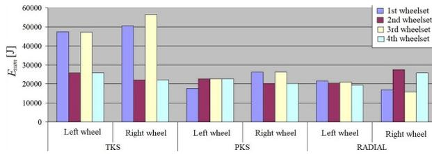
FIGURE 5. Total loss of mechanical energy  $E_{sum}$  [J] due to slipping of the tram wheels and the rails during the passage of the considered route at a speed of  $10 \text{ km}\cdot\text{h}^{-1}$ ; TKS – a bogie with the traditional construction scheme, PKS – a bogie with the perspective construction scheme, RADIAL – a bogie with the radial setting system.
