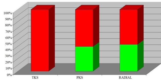
FIGURE 7. Possible effect of energy saving by using the innovative technical solutions at a running speed of  $10 \text{ km}\cdot\text{h}^{-1}$ : red colour – the amount of energy dissipated due to wheel slippage on the rails when the tram moves along the route, green colour – energy saving effect; TKS – a bogie with the traditional construction scheme, PKS – a bogie with the perspective construction scheme, RADIAL – a bogie with the radial setting system.
