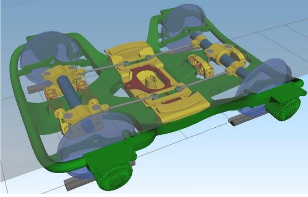
FIGURE 4. A scheme of a tram car running gear with a radial installation of wheelsets and with wheels of a standard design.
