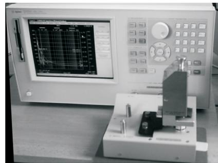
Fig. 9: Measurement system – the Agilent E4991A Material Analyzer
