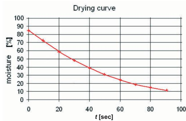
Fig. 13: Typical drying characteristic of this type applicator
