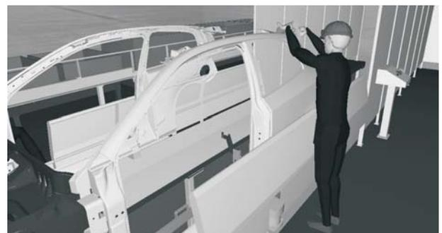
Fig. 4: The Smearing Sealer operation realized by the 5th percentile (on the left), vs the Smearing Sealer operation not practicable by the 5th percentile (on the right)
