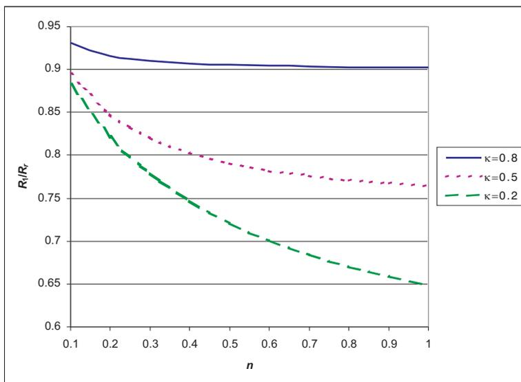
Fig. 2: Dependence of  $R_1/R_r$  on  $n$  for selected values of ratio  $\kappa$
