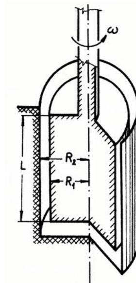
Fig. 1: Viscometer with coaxial cylinders
