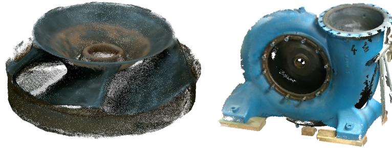
FIGURE 2. Cloud point of the runner (left) and the volute of the turbine (right).
