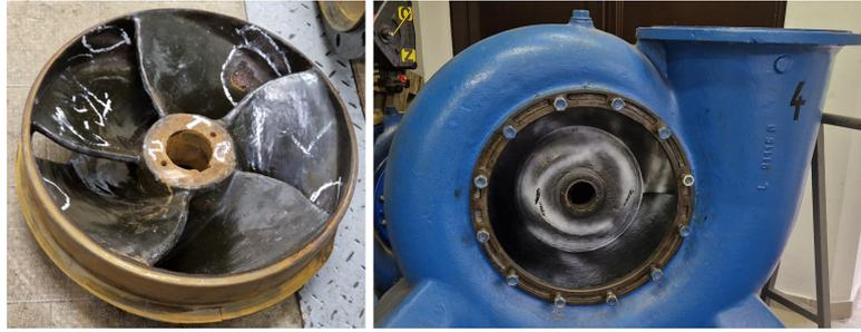
FIGURE 1. Original runner of the PAT (left) and the volute of the turbine (right).
