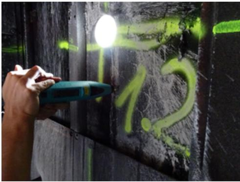
FIGURE 10. Rebound hammer test.
