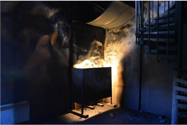
FIGURE 3. A gas burner partially covered by metal sheets.
