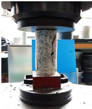
FIGURE 11. Concrete core destructive compressive strength test.
