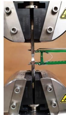
FIGURE 14. Steel yield strength test.
