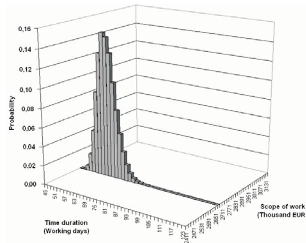
Fig. 3: Probability 3D bar chart for a construction project with fixed cost scope C
