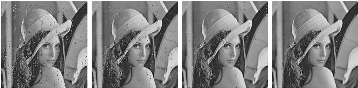
(B). P-LDPC coded at SNR = 4 dB and n = 1.1k (for 64-FFT, 128-FFT, 256-FFT, 512-FFT from left to right).
