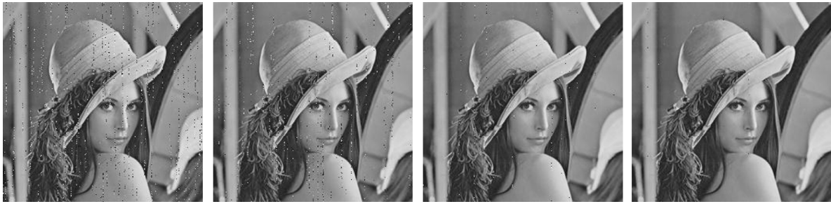
(A). P-LDPC coded at SNR = 3 dB and 128-FFT (for n = 1.1k, 2.3k, 4.6k, 9.2k from left to right).
