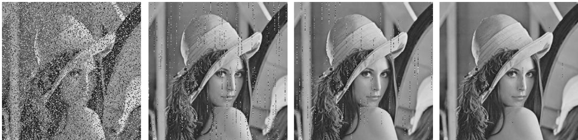
(c). Various coding schemes at SNR = 5 dB and n = 1.1k (for 2-D TPC, Polar SCL-4, Polar SCL-8, P-LDPC from left to right).
