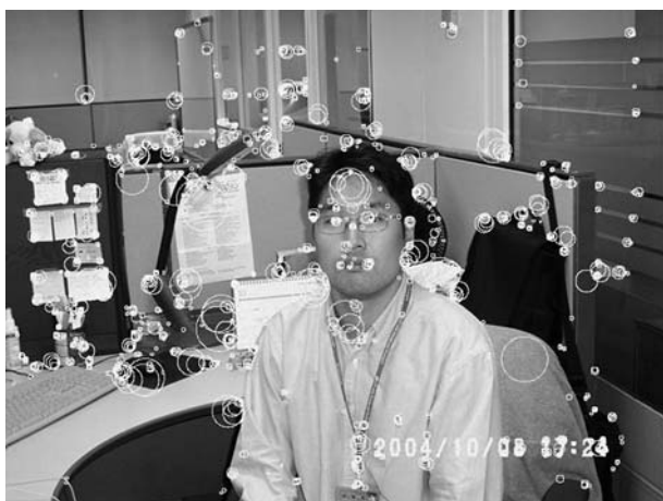
Fig. 7: This image of the test set shows all interest points detected by the scale-adapted Harris corner detector. The diameter of the circle indicates the appropriate scale on which the interest point has been detected.
