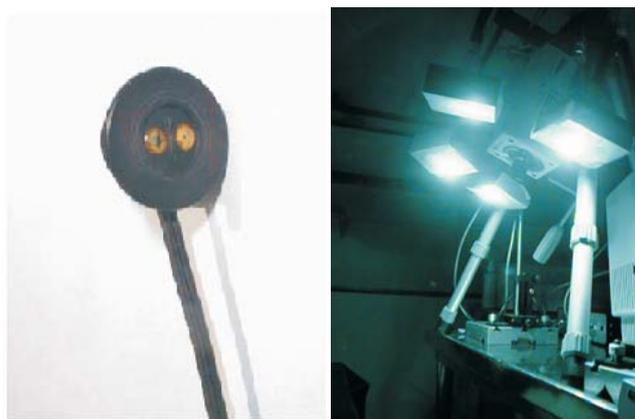
Fig. 6: PPG sensor (left) and PPGI camera with surrounding light sources (right)
