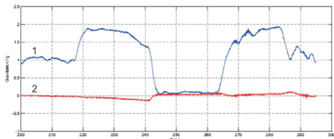
Fig. 5: Typical development of g-forces during a parabola maneuver (1: g-forces vertically, 2: g-forces in flight direction)
