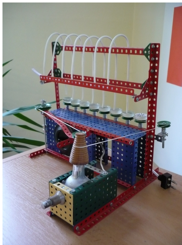
FIGURE 5. Merkur-based apparatus for centrifugal casting of contact lenses by Wichterle [29] (compare [30]).
