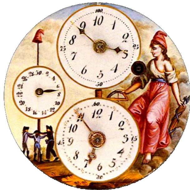
FIGURE 2. A demonstration of clocks with decimal time (top), traditional time (bottom) and a Republican Day in the thirty-day month (middle left) [16, p. 23].
