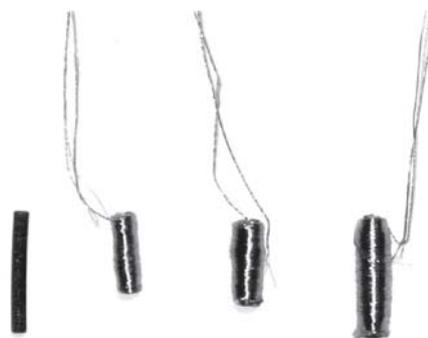
Fig. 6: Examples of bare coils made of self-bonding copper wire and a ferromagnetic core 8 mm in length. From the right 2000 turn coil, 1000 turn coil and 500 turn coil.
