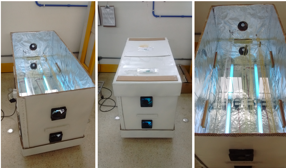
FIGURE 1. Low-cost equipment for UV exposure for fibres.
