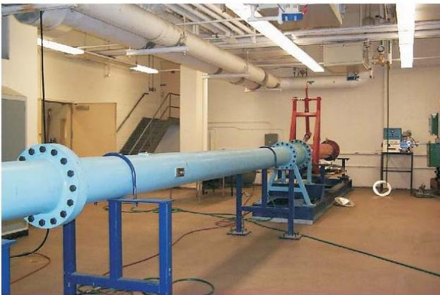
Fig. 1: Shock tube facility at CCNY, Driver section
